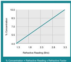
% Concentration = Refractive Reading x Refractive Factor Coolant Refractometer Factor % Brix = 3.0
