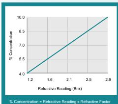
6 Concentration = Refractive Reading x Refractive Factor Coolant Refractometer Factor % Brix = 3.4
