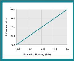
% Concentration = Refractive Reading x Refractive Factor Coolant Refractometer Factor % Brix = 2.0
