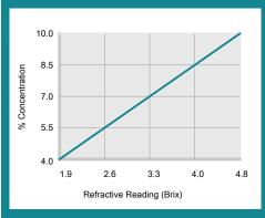
% Concentration = Refractive Reading x Refractive Factor Coolant Refractometer Factor % Brix = 2.1
