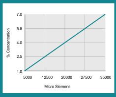
% Concentration = Conductivity in Micro Siemens x Factor Conductivity Factor = 0.00020
