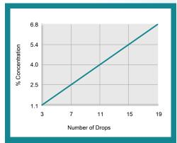
% Concentration = No. of Drops x Titration Factor Titration Factor = 0.36
