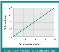
% Concentration = Refractive Reading x Refractive Factor Coolant Refractometer Factor % Brix = 3.4
