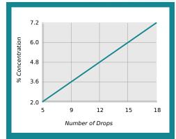
% Concentration = No. of Drops x Titration Factor Titration Factor = 0.40
