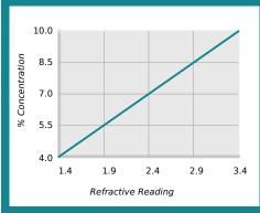
% Concentration = Refractive Reading x Refractive Factor Coolant Refractometer Factor % Brix = 2.9
